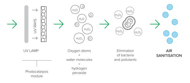
\*Diagram of a generic photocatalysis process (by way of an example).
